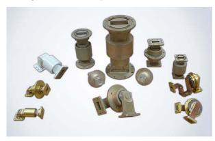
1.70 - 22.00 GHz Performance Frequency1.25 Typical Max VSWR (VSWR varies with design)Numerous Flange Configurations availableAluminum (6061) or Copper WR Waveguide Available
